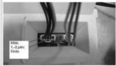
Picture F13-4: 5Vdc Control on KN4 socket on the motor card
