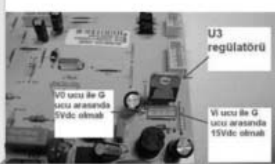
Picture F13-6: 15Vdc control between the Vi and G ends of the U3 regulator on motor card, and 5Vdc control between G and V0 ends
