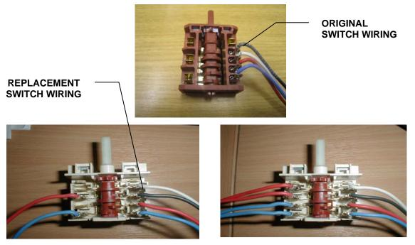
Failure to reverse the black and white wire connections will result in the hotplate not regulating correctly.
