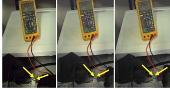
• Check the thermostat from the terminals. If manual resetting thermostat is open curcuit, the button is up and the heater does not work. Then push the button down, and measure the thermostat to be sure that it is short circuit.
