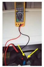
$\boldsymbol{\cdot}$  Check the resistance value between NTC and housing from the socket, It should be open circuit.
