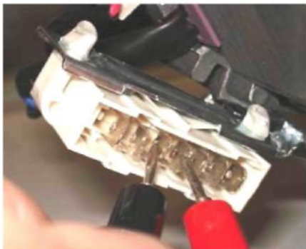
PICTURE E11-5: Motor rotor is being controlled over 8-pin motor
